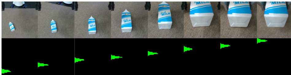
Figure 6: Demonstration of our trained value function on a successful trajectory. In the distribution (second row), we visualize the outputs of the value function through a successful trajectory. The value function distribution increases as the robot gets closer to the milk jug. The value function learns a distance to task completion by images alone.
